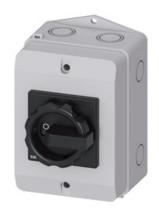
SENTRON, Switch disconnector 3LD, main switch, 4-pole, 25 A, Operating power at AC- 23 A at 400 V: 9.5 kW, molded-plastic encapsulation for metric cable gland, rotary operating mechanism, black
