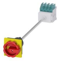
SENTRON, Switch disconnector 3LD, emergency switching-off switch, 4-pole, lu: 16 A, operating power / at AC-23 A 400 V: 7.5 kW, floor mounting with door coupling, rotary operating mechanism, Red / yellow, 4-hole mounting of the handle
