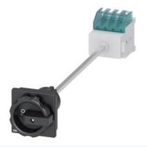
SENTRON, Switch disconnector 3LD, main switch, 3-pole, lu: 16 A, Operating power / at AC-23 A at 400 V: 7.5 kW, floor mounting with door coupling, rotary operating mechanism, black, 4-hole mounting of the handle, without tolerance compensation
