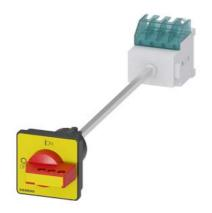
SENTRON, switch disconnector 3LD, EMERGENCY OFF switch, 3-pole, lu: 16 A, Operating power / at AC-23 A at 400 V: 7.5 kW, floor mounting with door coupling, defeatable knob-operated mechanism, red/yellow, 4-hole mounting of the handle
