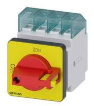
SENTRON, Switch disconnector 3LD, emergency switching-off switch, 3-pole, Iu: 16 A, operating power / at AC-23 A 400 V: 7.5 kW, front-mounted, knob-operated mechanism, red/yellow, 4-hole mounting of the handle
