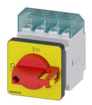
SENTRON, Switch disconnector 3LD, emergency switching-off switch, 4-pole, Iu: 16 A, operating power / at AC-23 A 400 V: 7.5 kW, front-mounted, knob-operated mechanism, red/yellow, 4-hole mounting of the handle
