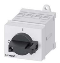
SENTRON, Switch disconnector 3LD, main switch, 4-pole, lu: 16 A, Operating power / at AC-23 A at 400 V: 7.5 kW, installation in distribution boards, knob-operated mechanism, black, handle direct at the switch
