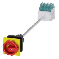
SENTRON, Switch disconnector 3LD, emergency switching-off switch, 3-pole, Iu: 16 A, operating power / at AC-23 A 400 V: 7.5 kW, floor mounting with door coupling, rotary operating mechanism, Red / yellow, central mounting 22.5 mm of the handle
