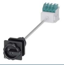
SENTRON, Switch disconnector 3LD, main switch, 4-pole, lu: 16 A, Operating power / at AC-23 A at 400 V: 7.5 kW, floor mounting with door coupling, rotary operating mechanism, black, central mounting 22.5 mm of the handle
