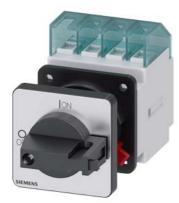
SENTRON, Switch disconnector 3LD, main switch, 4-pole, lu: 16 A, Operating power / at AC-23 A at 400 V: 7.5 kW, front-mounted, knob-operated mechanism, black, central mounting 22.5 mm of the handle
