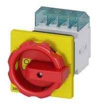
SENTRON, Switch disconnector 3LD, emergency switching-off switch, 3-pole, lu: 16 A, operating power / at AC-23 A 400 V: 7.5 kW, front-mounted, rotary operating mechanism, Red / yellow, central mounting 22.5 mm of the handle
