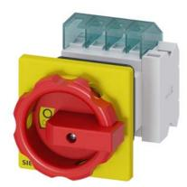
SENTRON, Switch disconnector 3LD, emergency switching-off switch, 3pole, Iu: 16 A, operating power / at AC-23 A 400 V: 7.5 kW, front-mounted, 1 NC, 1 NO, rotary operating mechanism, Red / yellow, Central mounting 22.5 mm of the handle
