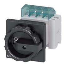
SENTRON, Switch disconnector 3LD, main switch, 4-pole, lu: 16 A, Operating power / at AC-23 A at 400 V: 7.5 kW, front-mounted, 1 NC, 1 NO, rotary operating mechanism, black, Central mounting 22.5 mm of the handle
