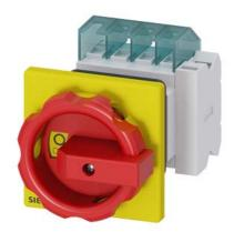
SENTRON, Switch disconnector 3LD, emergency switching-off switch, 4-pole, lu: 16 A, operating power / at AC-23 A 400 V: 7.5 kW, front-mounted, 1 NC, 1 NO, rotary operating mechanism, Red / yellow, Central mounting 22.5 mm of the handle
