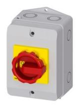
SENTRON, Switch disconnector 3LD, emergency switching-off switch, 3-pole, lu: 16 A, operating power / at AC-23 A 400 V: 7.5 kW, Molded plastic encapsulation for metric cable gland, rotary operating mechanism, red/yellow
