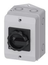
SENTRON, Switch disconnector 3LD, main switch, 3-pole, lu: 16 A, Operating power / at AC-23 A at 400 V: 7.5 kW, molded-plastic encapsulation for metric screw connection, 1 NC, 1 NO, rotary operating mechanism, black
