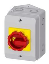
SENTRON, Switch disconnector 3LD, emergency switching-off switch, 3-pole, lu: 16 A, operating power / at AC-23 A 400 V: 7.5 kW, Molded plastic encapsulation for metric cable gland, 1 NC, 1 NO, rotary operating mechanism, red/yellow
