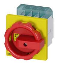
SENTRON, Switch disconnector 3LD, emergency switching-off switch, 4-pole, lu: 16 A, operating power / at AC-23 A 400 V: 7.5 kW, front-mounted, rotary operating mechanism, Red / yellow, 4-hole mounting of the handle
