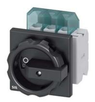
SENTRON, Switch disconnector 3LD, main switch, 3-pole, lu: 25 A, Operating power / at AC-23 A at 400 V: 9.5 kW, front-mounted, 1 NC, 1 NO, rotary operating mechanism, black, 4-hole mounting of the handle
