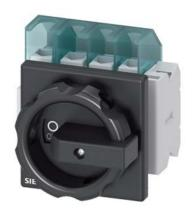
SENTRON, Switch disconnector 3LD, main switch, 4-pole, lu: 25 A, Operating power / at AC-23 A at 400 V: 9.5 kW, front-mounted, 1 NC, 1 NO, rotary operating mechanism, black, 4-hole mounting of the handle
