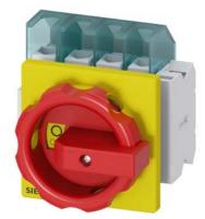
SENTRON, Switch disconnector 3LD, emergency switching-off switch, 4-pole, Iu: 25 A, operating power / at AC-23 A 400 V: 9.5 kW, front-mounted, 1 NC, 1 NO, rotary operating mechanism, Red / yellow, 4-hole mounting of the handle
