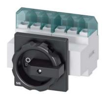
SENTRON, Switch disconnector 3LD, main switch, 6-pole, lu: 25 A, Operating power / at AC-23 A at 400 V: 9.5 kW, front-mounted, rotary operating mechanism, black, 4-hole mounting of the handle
