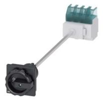
SENTRON, Switch disconnector 3LD, main switch, 4-pole, lu: 25 A, Operating power / at AC-23 A at 400 V: 9.5 kW, floor mounting with door coupling, rotary operating mechanism, black, 4-hole mounting of the handle
