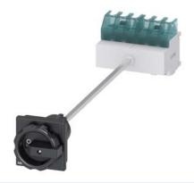
SENTRON, Switch disconnector 3LD, main switch, 6-pole, lu: 25 A, Operating power / at AC-23 A at 400 V: 9.5 kW, floor mounting with door coupling, rotary operating mechanism, black, 4-hole mounting of the handle
