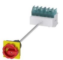
SENTRON, Switch disconnector 3LD, emergency switching-off switch, 6pole, lu: 25 A, operating power / at AC-23 A 400 V: 9.5 kW, floor mounting with door coupling, rotary operating mechanism, Red / yellow, 4-hole mounting of the handle
