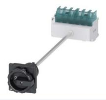
SENTRON, Switch disconnector 3LD, main switch, 6-pole, lu: 25 A, Operating power / at AC-23 A at 400 V: 9.5 kW, floor mounting with door coupling, 1 NC, 1 NO, rotary operating mechanism, black, 4-hole mounting of the handle
