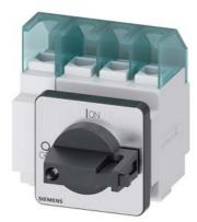
SENTRON, Switch disconnector 3LD, main switch, 4-pole, lu: 25 A, Operating power / at AC-23 A at 400 V: 9.5 kW, floor mounting with door coupling, knob-operated mechanism, black, 4-hole mounting of the handle
