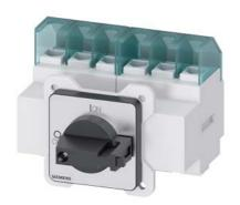
SENTRON, Switch disconnector 3LD, main switch, 6-pole, lu: 25 A, Operating power / at AC-23 A at 400 V: 9.5 kW, floor mounting with door coupling, knob-operated mechanism, black, 4-hole mounting of the handle
