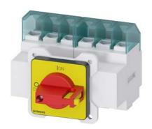
SENTRON, Switch disconnector 3LD, emergency switching-off switch, 6-pole, lu: 25 A, operating power / at AC-23 A 400 V: 9.5 kW, floor mounting with door coupling, knob-operated mechanism, red/yellow, 4-hole mounting of the handle, in neutral position can be locked
