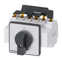
SENTRON, Switch disconnector 3LD, change-over switch, 3-pole, lu: 25 A, Operating power / at AC-23 A at 400 V: 9.5 kW, Front mounting, knob-operated mechanism, black, 4-hole mounting of the handle
