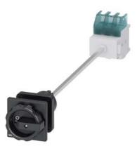
SENTRON, Switch disconnector 3LD, main switch, 3-pole, lu: 25 A, Operating power / at AC-23 A at 400 V: 9.5 kW, floor mounting with door coupling, rotary operating mechanism, black, central mounting 22.5 mm of the handle
