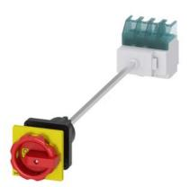
SENTRON, Switch disconnector 3LD, emergency switching-off switch, 4-pole, Iu: 25 A, operating power / at AC-23 A 400 V: 9.5 kW, floor mounting with door coupling, rotary operating mechanism, Red / yellow, central mounting 22.5 mm of the handle
