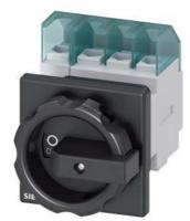
SENTRON, Switch disconnector 3LD, main switch, 4-pole, lu: 25 A, Operating power / at AC-23 A at 400 V: 9.5 kW, front-mounted, rotary operating mechanism, black, central mounting 22.5 mm of the handle
