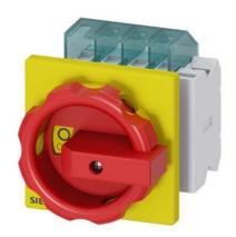
SENTRON, Switch disconnector 3LD, emergency switching-off switch, 4-pole, lu: 16 A, operating power / at AC-23 A 400 V: 7.5 kW, front-mounted, 1 NC, 1 NO, rotary operating mechanism, Red / yellow, 4-hole mounting of the handle
