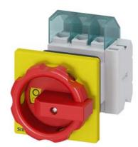
SENTRON, Switch disconnector 3LD, emergency switching-off switch, 3-pole, lu: 25 A, operating power / at AC-23 A 400 V: 9.5 kW, front-mounted, 1 NC, 1 NO, rotary operating mechanism, Red / yellow, Central mounting 22.5 mm of the handle
