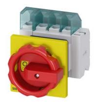
SENTRON, Switch disconnector 3LD, emergency switching-off switch, 4-pole, Iu: 25 A, operating power / at AC-23 A 400 V: 9.5 kW, front-mounted, 1 NC, 1 NO, rotary operating mechanism, Red / yellow, Central mounting 22.5 mm of the handle
