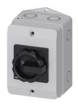
SENTRON, Switch disconnector 3LD, main switch, 3-pole, lu: 25 A, Operating power / at AC-23 A at 400 V: 9.5 kW, molded-plastic encapsulation for metric cable gland, rotary operating mechanism, black
