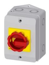
SENTRON, Switch disconnector 3LD, emergency switching-off switch, 3-pole, lu: 25 A, operating power / at AC-23 A 400 V: 9.5 kW, Molded plastic encapsulation for metric cable gland, rotary operating mechanism, red/yellow
