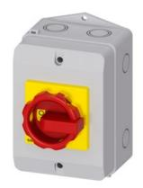
SENTRON, Switch disconnector 3LD, emergency switching-off switch, 3-pole, lu: 25 A, operating power / at AC-23 A 400 V: 9.5 kW, Molded plastic encapsulation for metric cable gland, 1 NC, 1 NO, rotary operating mechanism, red/yellow
