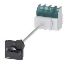
SENTRON, switch disconnector 3LD, main switch, 4-pole, lu: 63 A, operating power / at AC-23 A at 400 V: 22 kW, floor mounting with door coupling, defeatable knob-operated mechanism, black, 4-hole mounting of the handle
