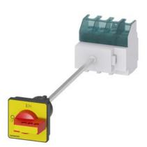
SENTRON, switch disconnector 3LD, EMERGENCY OFF switch, 4-pole, lu: 63 A, Operating power / at AC-23 A at 400 V: 22 kW, floor mounting with door coupling, defeatable knob-operated mechanism, red/yellow, 4-hole mounting of the handle
