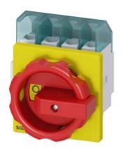
SENTRON, Switch disconnector 3LD, emergency switching-off switch, 4-pole, lu: 32 A, operating power / at AC-23 A 400 V: 11.5 kW, front-mounted, rotary operating mechanism, Red / yellow, 4-hole mounting of the handle
