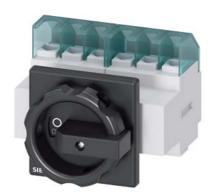
SENTRON, Switch disconnector 3LD, main switch, 6-pole, lu: 32 A, Operating power / at AC-23 A at 400 V: 11.5 kW, front-mounted, rotary operating mechanism, black, 4-hole mounting of the handle
