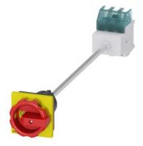
SENTRON, Switch disconnector 3LD, emergency switching-off switch, 3-pole, Iu: 32 A, operating power / at AC-23 A 400 V: 11.5 kW, floor mounting with door coupling, rotary operating mechanism, Red / yellow, 4-hole mounting of the handle
