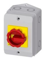
SENTRON, Switch disconnector 3LD, emergency switching-off switch, 4pole, 25 A, operating power at AC-23 A at 400 V: 9.5 kW, molded-plastic encapsulation for metric cable gland, rotary operating mechanism, red/yellow
