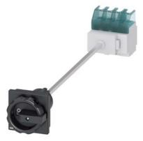
SENTRON, Switch disconnector 3LD, main switch, 4-pole, lu: 32 A, Operating power / at AC-23 A at 400 V: 11.5 kW, floor mounting with door coupling, rotary operating mechanism, black, 4-hole mounting of the handle
