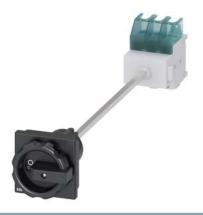
SENTRON, Switch disconnector 3LD, main switch, 3-pole, lu: 32 A, Operating power / at AC-23 A at 400 V: 11.5 kW, floor mounting with door coupling, rotary operating mechanism, black, 4-hole mounting of the handle, without tolerance compensation
