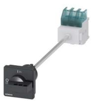
SENTRON, switch disconnector 3LD, main switch, 3-pole, lu: 32 A, operating power / at AC-23 A at 400 V: 11.5 kW, floor mounting with door coupling, defeatable knob-operated mechanism, black, 4-hole mounting of the handle
