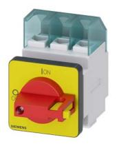
SENTRON, Switch disconnector 3LD, emergency switching-off switch, 3-pole, lu: 32 A, operating power / at AC-23 A 400 V: 11.5 kW, front-mounted, knob-operated mechanism, red/yellow, 4-hole mounting of the handle
