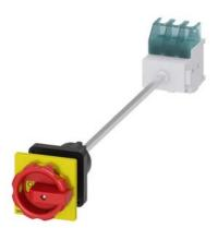
SENTRON, Switch disconnector 3LD, emergency switching-off switch, 3-pole, Iu: 32 A, operating power / at AC-23 A 400 V: 11.5 kW, floor mounting with door coupling, rotary operating mechanism, Red / yellow, central mounting 22.5 mm of the handle
